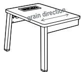
On surface power module on narrow tables
