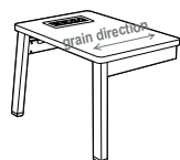
On surface power module on narrow tables
