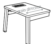
On surface power module on narrow tables
